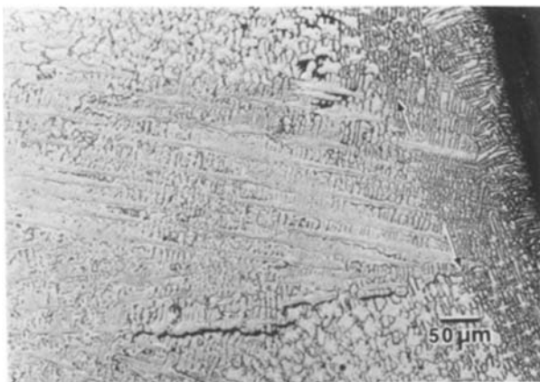
Figure 3 Optical micrograph of weld microstructure at the quench interface (arrows), Heat 1.
